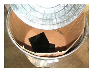
Cut pieces of your insulating material for the bottom and to go around the sides of the trash can, on the inside. It is not absolutely necessary, but it's a good idea to tape or glue them in
